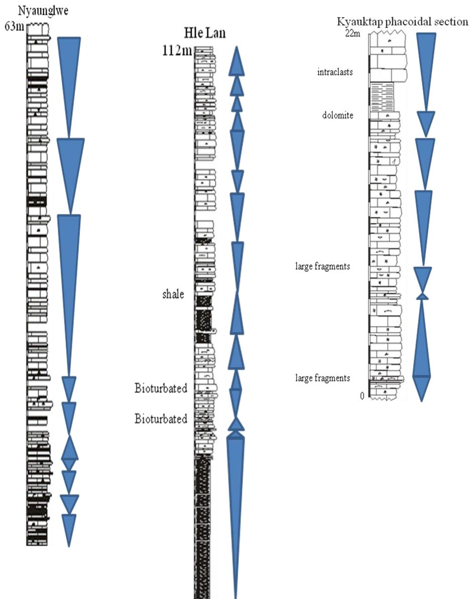
**Figure 4:** Vertical stacking pattern of deposition in three sections
